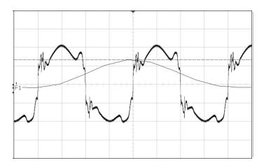
Figure 6 - LPS voltage waveform (units are arbitrary) ): periodicity is  $50~\rm{Hz}$ , while the amplitude was scaled using the voltage divider.
