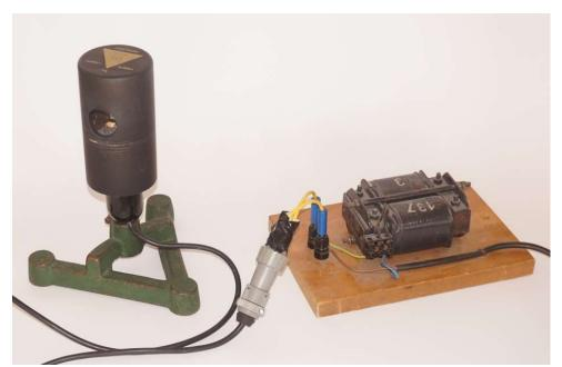
Figure 1 - Leybold 45115 High Pressure Mercury Lamp and in-house matched choke. Luminance 600 cd/cm $^2$ , CCT  $\sim$  6000 K, operating current  $\sim$  1 A.
