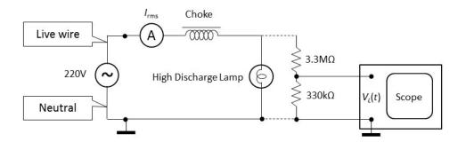
Figure 2 - Measurement of the lamp voltage fundamental harmonic. Voltage divider is used to reduce the voltage seen by the oscilloscope and for this purpose one must track the live and neutral lines.
