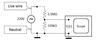
Figure 4 - Measurement of the main power voltage. Voltage divider is used to reduce the voltage seen by the oscilloscope and for this purpose one must track the live and neutral lines.
