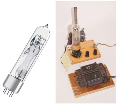
Figure 2 - OSRAM Na/10 Low-pressure sodium spectral lamp with choke and starter.
