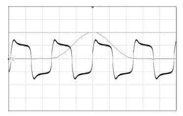
Figure 5 - HPM voltage waveform (units are arbitrary): periodicity is 50 Hz, while the amplitude was scaled using the voltage divider.
