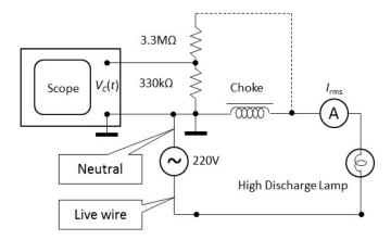
Figure 3 - Measurement of the choke voltage. Voltage divider is used to reduce the voltage seen by the oscilloscope and for this purpose one must track the live and neutral lines.
